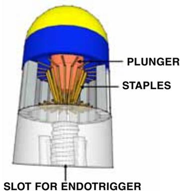
**Figure 3 | Diagram depicting the head with titanium staples arranged around the plunger. When the plunger is pulled forward the staples are displaced outward.**
