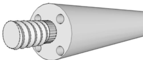
**Figure 4 | Distal end of the endo-trigger has two types of ports, a central port to connect to the head, and another to pull the plunger.**
