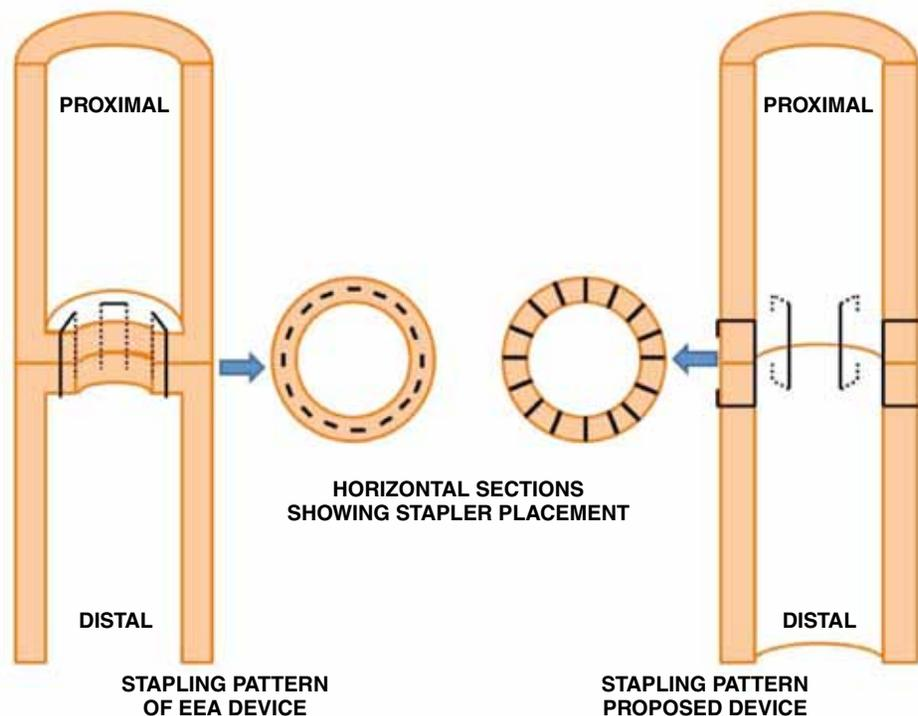
**Figure 8 | Sagittal and horizontal sections of the esophagus showing placement of staples in conventional EEA and the proposed device.** Conventional EEA places staples with the body of the staple perpendicular to the long axis of the esophagus limiting future growth. The proposed stapler device would place the staples with their body parallel to the long axis of the esophagus. Thus it would not impede future growth.
