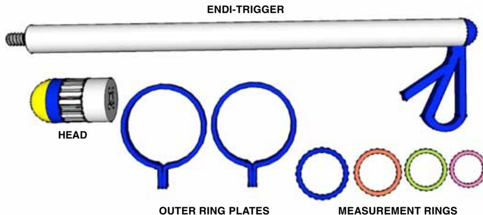
**Figure 2 | Schematic showing the components of the stapler device—the head, endo-trigger, outer ring plates and measurement rings.**
