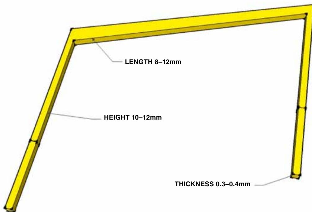
**Figure 5 | Dimensions of Titanium Staples**
