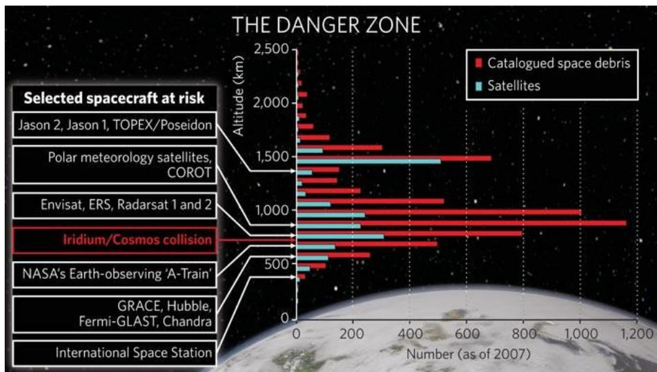
**Figure 2 | Levels of space debris as of 2007.** Orbits with more space debris have higher risks of impact. Space debris in higher orbits requires the most time to fall back to Earth. Reproduced with permission from G. Forden, Massachusetts Institute of Technology.
